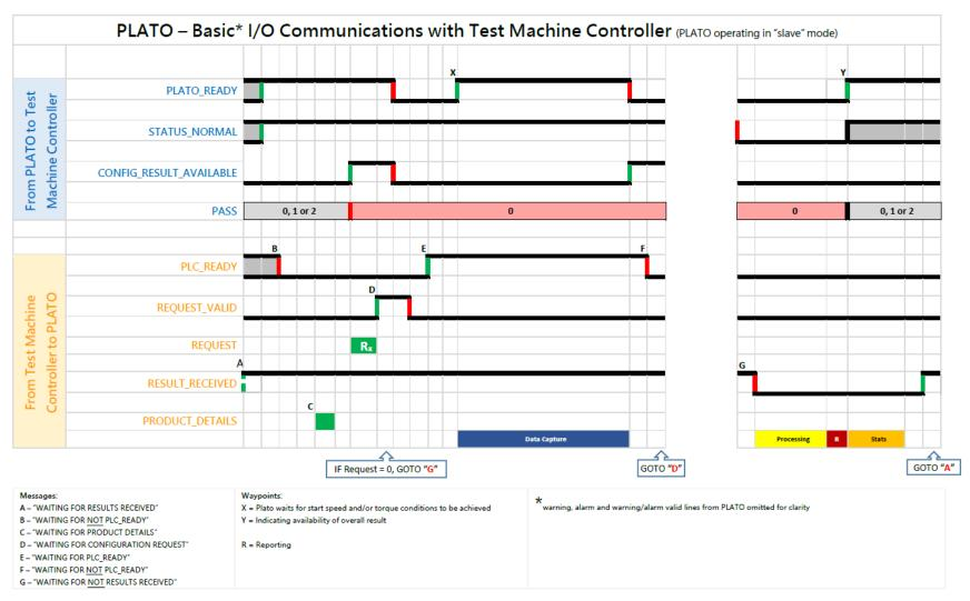
SYSTEM OK (Plato to TMC\*) will remain HIGH under normal operation. If LOW sensed by TMC\*, Plato is indicating an error and testing cannot proceed. Retest functionality via RETEST (Plato to TMC\*) not covered by above.
