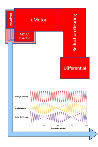
Although eMotor/ePowertrain NVH testing can be accomplished using speed reference from <u>both output shafts</u>, a higher speed eMotor reference signal is preferable.
