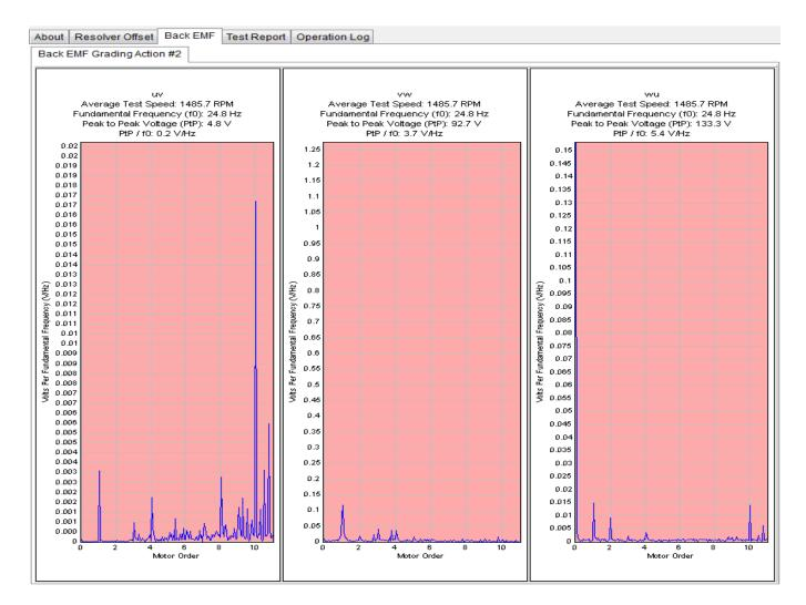
Results are then summarised in the usual PLATO html-format test report and, if required, transmitted to the test machine controller (PLC) via OPC for display on the machine's HMI etc. By default, pass/fail limits may be placed on the fundamental rotation order plus harmonics thereof up to x10. Excessive harmonic levels can be an indication of poor winding quality. Red/green shading provides a clear indication of features that have passed/failed.
